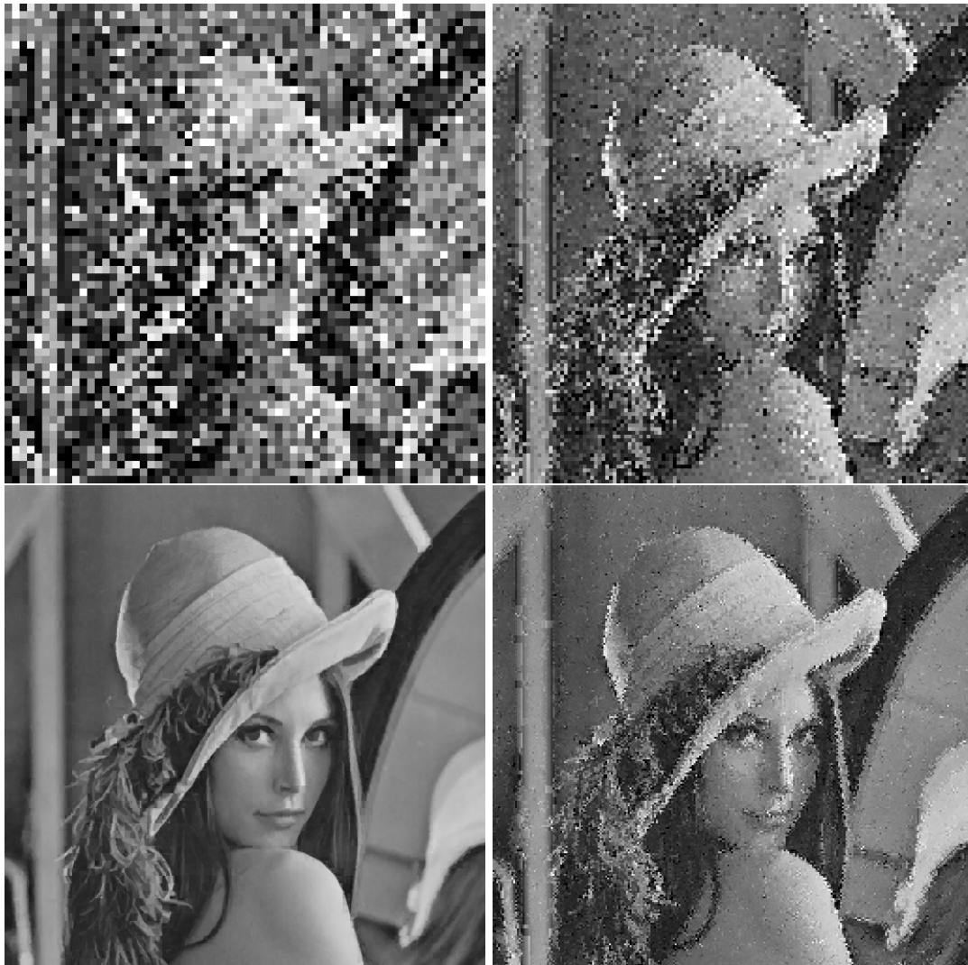
Figure 12. Starting at upper left and moving clockwise: The iterates u_1 , u_2 , and u_3 along with the fixed point \bar{u} of the fractal transform operator T designed to approximate the standard 512 \times 512 (8 bits/pixel) Lena image. The “seed” image was u_0(x) = 255 (plain white). The fractal transform T was obtained by “collage coding” using 4096 8 \times 8 nonoverlapping pixel range blocks. The domain pool consisted of the set of 1024 nonoverlapping 16 \times 16 pixel blocks.
