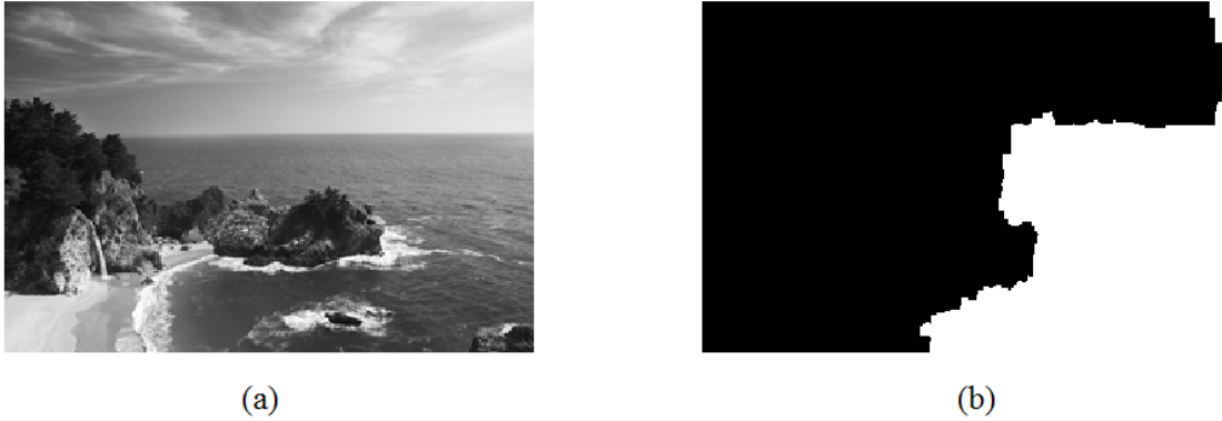
Figure 1.10: The graph cut provided in the source code. (a) The original image. (b) The resulting segmentation B = [B_1, B_2, \dots, B_N] where B_k \forall k = 1, 2, \dots, N are either 1 (“s object”) or 2 (“t background”) provided that N is the total number of pixels.
